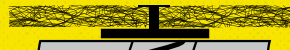
Type 3 W Special belt joint for non-woven web belts. Tape reinforced butt joint with additional frontal adhesion.
