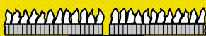
Type 3 G Zig zag joint, with cloth-reinforced foil backing, impact-free working at very sensitive parts, in particular glass.
